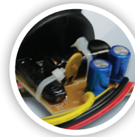
Built-In Overload Protection Circuit
